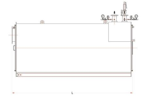
Heater for hot water, coil type
