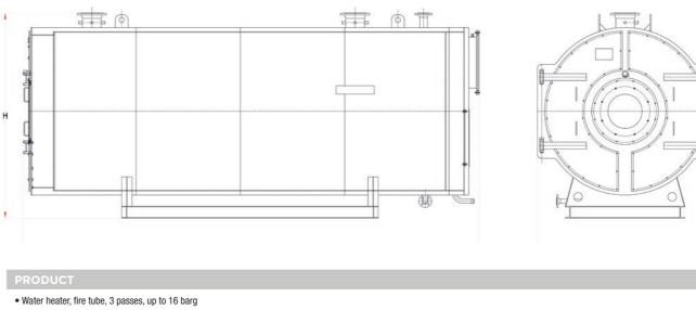
• Fire tube • 3 passes • Wet back • Through furnace • Horizontal
