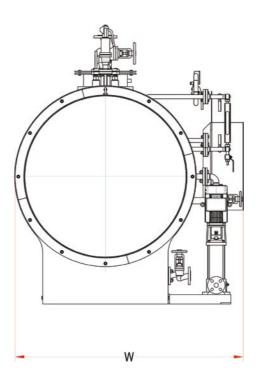
• Steam generators, fire tube, 2 passes, up to 18 barg
