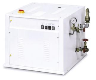
Electric and automatic steam generator, available with variable power from 15 to 180 kW, made with one or more electrical resistors. Project pressure up to 10 barg. The MAXI generator can produce from a minimum of 9 Kg/h to a maximum of 170 Kg/h of steam at an operating pressure of 7 + 8 barg. It can be supplied directly from the water net or from a special stainless-steel tank.
