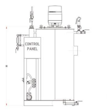
Tubeless steam generators Tubeless • 2 passes • Dry-back • Vertical • 50 kg/h - 500 kg/h
