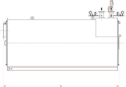
• Heater for superheated water, coil type
